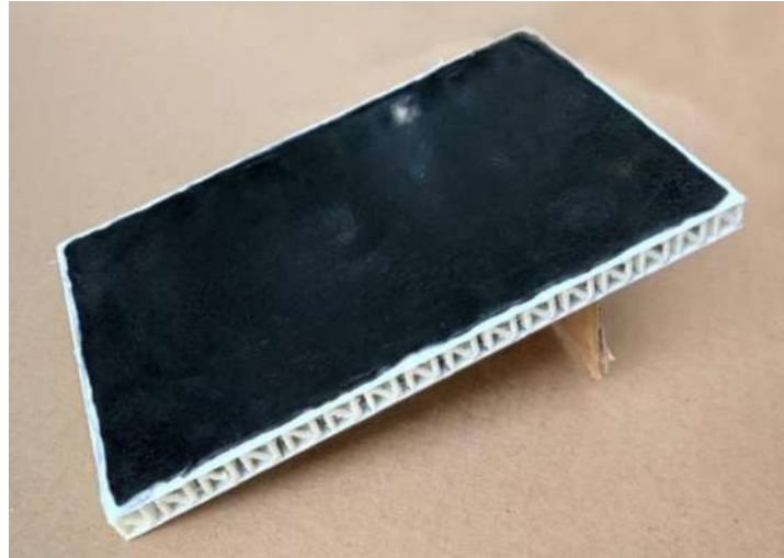
Figure 4: Sample 6 Prepared for the Strain Gauge Testing
